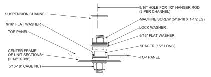
FIGURE 12 - DETAILS FOR SECURING SUSPENSION CHANNELS
